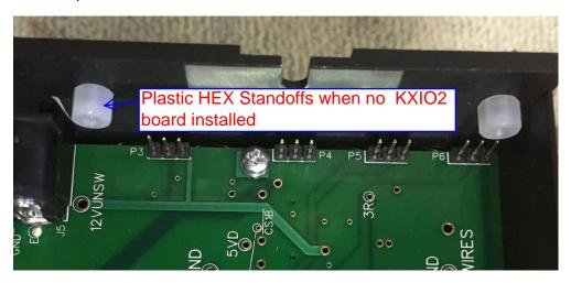
Place the KX2 with the removed end panel up, set the new Side KX end panel in place and start the top (2) Screws back into their corresponding holes. If you have the KXIO2 board align and start these mounting screws. You can now snug these screws down being careful not to over tighten them.
